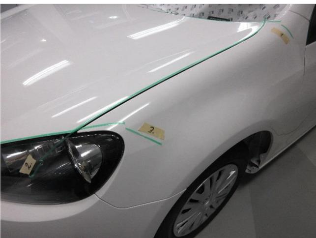
Repress the 3M™ Knifeless™ Tape to achieve a good bond to the substrate.
