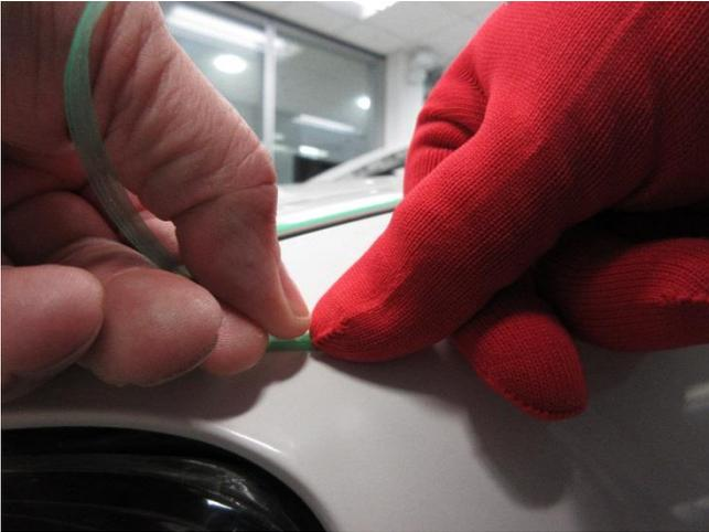
Gently pull the line to tear the carrier tape and expose the filament. Tack end of filament to vehicle until ready to cut film.
