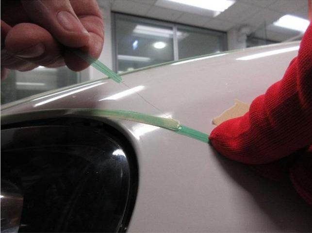
Fold the filament over the Cover Tape and press your thumb on it.
