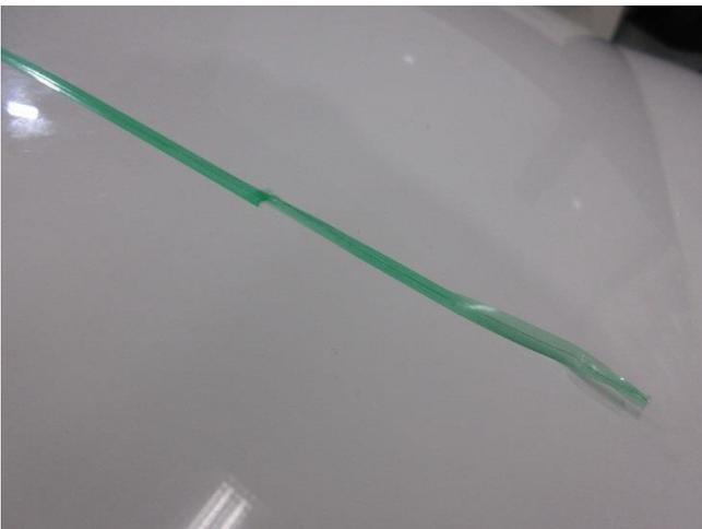
Apply the film with firm pressure over the tape, leaving the lead and tail tape visible.
