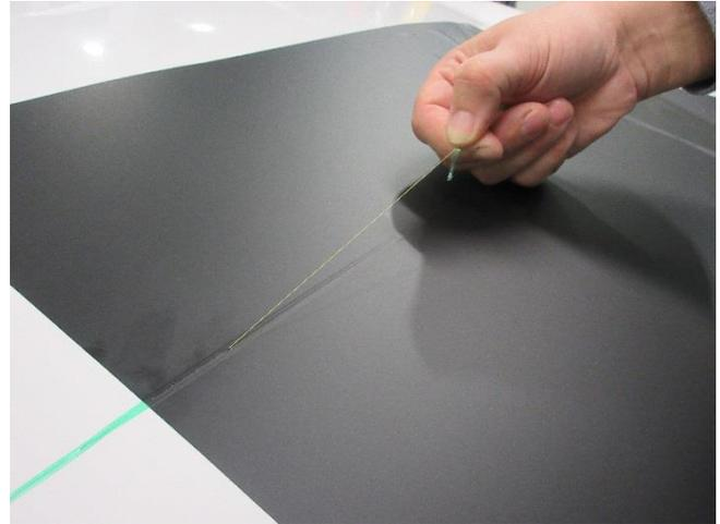
After cutting is finished, remove the excess film and the carrier tape from under the film. Please note that after cutting the carrier tape has split in two tapes. Both tapes need to be removed completely without residuals.
