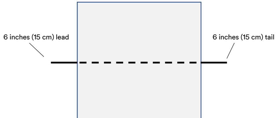
Begin with 6 inches (15 cm) of tape (before and after) where the graphic will be cut and lay down 3M™ Knifeless™ Tape. Apply the film with pressure over the 3M™ Knifeless™ Tape, leaving the lead and tail tape visible.
